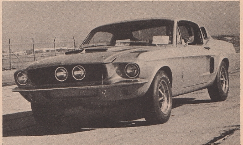
Top line GT-500 gets its go from a 428 hydraulic lifter engine with dual quads, aluminum rocker covers and dual exhausts. Off-the-line performance is good if car is ordered with Detroit Auto locker which is the only limited-slip unit available from Shelby American.
